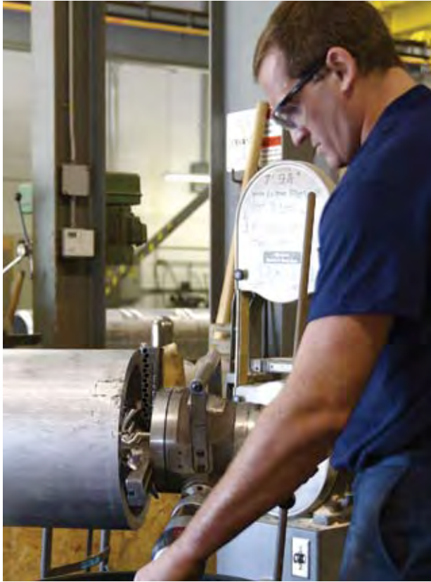
Welder/fabricator Wayne Bryant uses a portable lathe to finish the end of a segment of pipe at Gilchrist Metal Fabricating Company.
