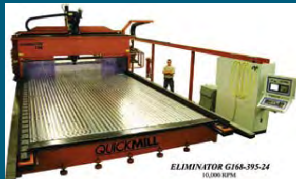
The Quickmill Eliminator G168-395-24 gantry-type machining center has a table 168" wide and 385" long.
