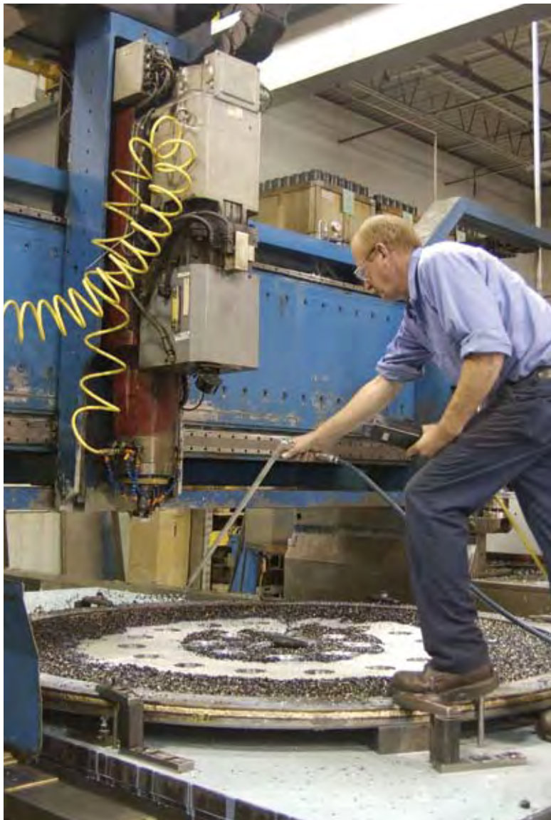
Machinist Dana Hamlin clears chips from the large disk he is machining on a Quickmill gantry-type machining center at Gilchrist Metal Fabricating Company.
