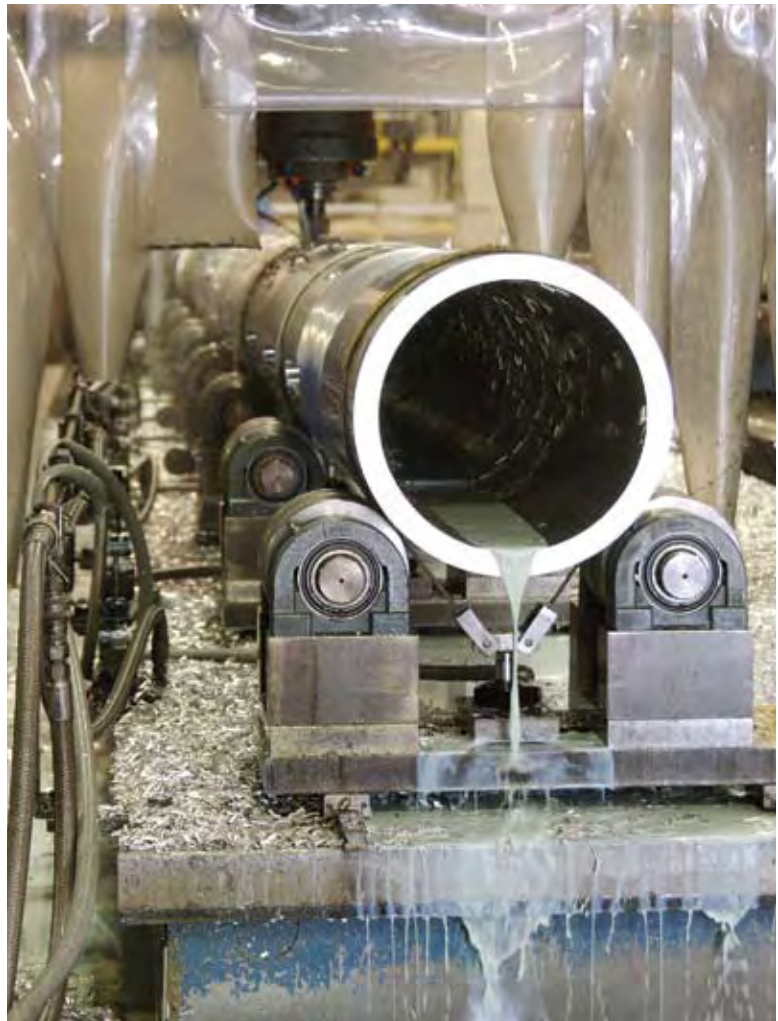
The hold-down system allows rotation of this hollow cylindrical workpiece at Gilchrist Metal Fabricating Company.
